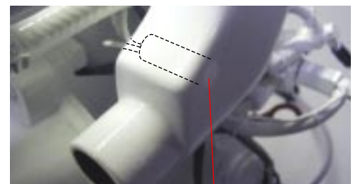
Exhaust Temperature Switch
