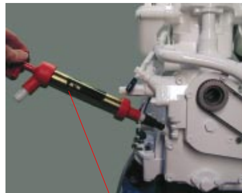
Dipstick Oil Pump
