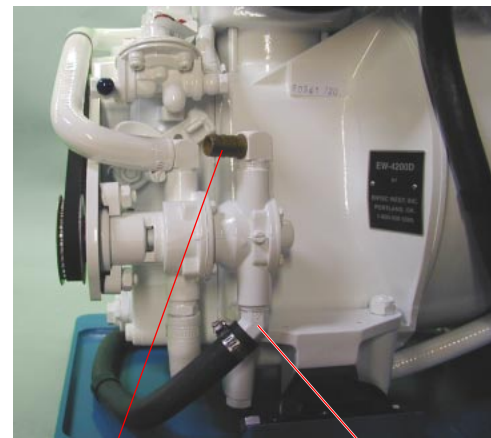
Raw Water Inlet
